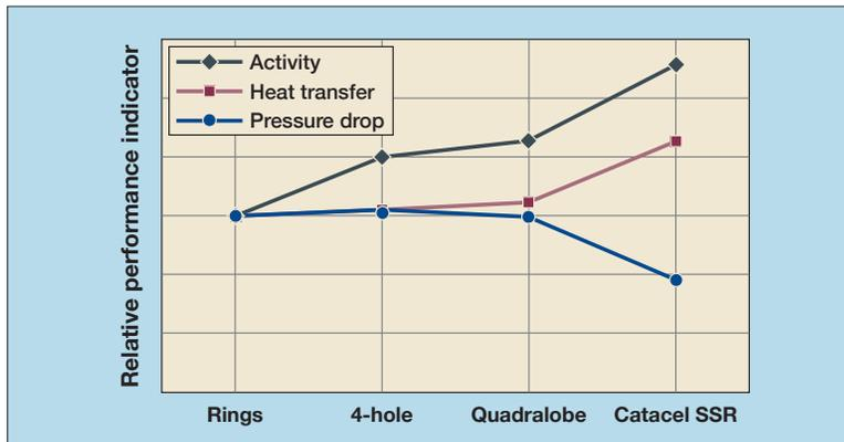
Figure 4 Relative performances of various steam reforming catalysts
