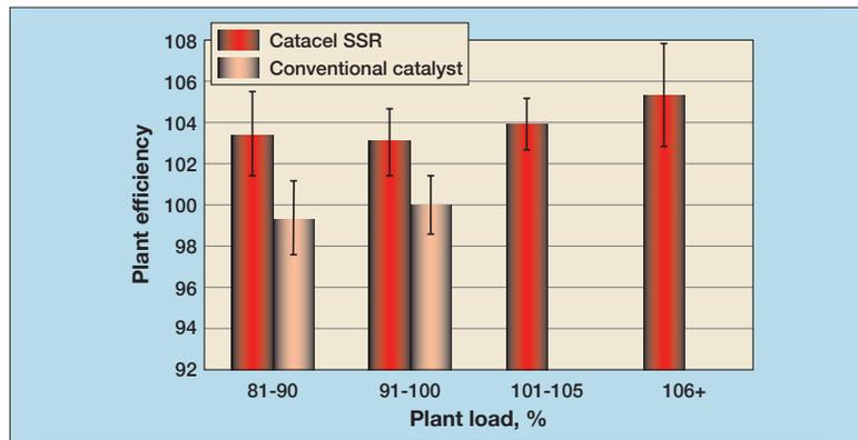
Figure 7 Plant efficiency (syngas flow/total natural gas flow) at various loads
