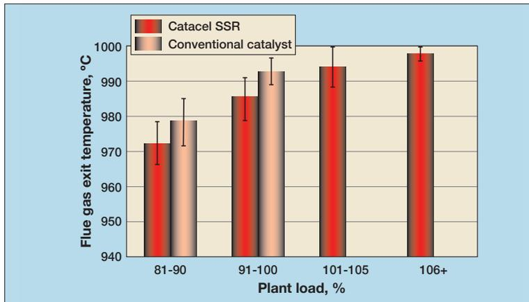
**Figure 6** Comparison of flue gas exit temperature for various plant loads
